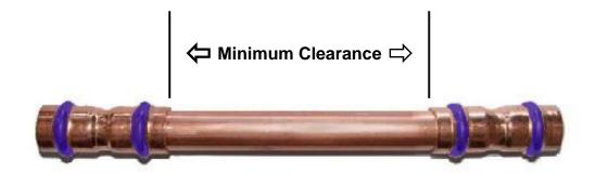
When an EZIPRESS™ fitting is being installed close to an existing brazed fitting, the clearances in the following table need to be observed. This will ensure that the press fitting is kept clear of tube that may have been excessively annealed during the brazing process.
