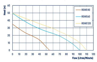
**POWER 240V** RATED MAXIMUM **INLET | OUTLET** SIZE L X W X H (MM) SUCTION NO. OF WEIGHT MODEL LIFT (M) CODE P2 FLOW HEAD FLOW (kW) (L/MIN) (M) (L/MIN) TAPS (KG) P1 (kW) HEAD AMPS MM IN (M) 22139 RSWE40 2.6 0.6 0.44 20 22 55 35 9 2-4 25 1" 10 380x180x195 9 1" 420x180x210 20548 RSWE60 4.6 0.98 0.74 40 29 100 49.5 4-7 25 15.7 1" 26359 RSWE120 5.7 1.26 0.88 60 29 110 49.7 9 5-8 25 16.2 420x180x210
