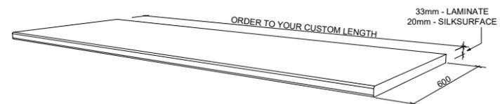
MAX LAMINATE BENCHTOP LENGTH = 3600mm | MAX SILKSURFACE BENCHTOP LENGTH = 3000mm
